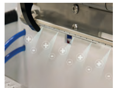
Ionizer bar to combat static electricity
